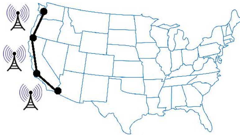
Figure 5.3: Illustration of a matching feasibility constraint. The players are broadcast stations seeking to buy radio spectrum, depicted as edges of a line graph along the U.S. coastline. A player set is infeasible if it contains players that are adjacent in the graph because they interfere with each other's broadcasts. A feasible set thus corresponds to a matching.
